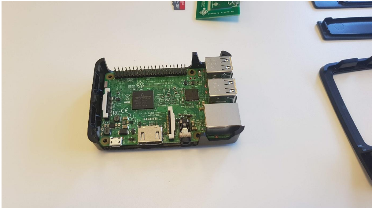
Figure 2. Attach the Raspberry PI Card on the case back-plate
