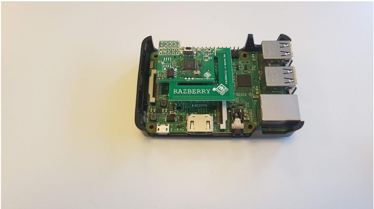
Figure 3. Connect the Z Wave Antenna to the Raspberry PI Pin Header
