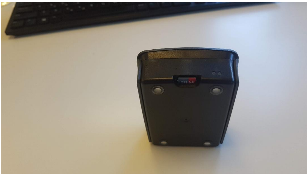
Figure 8. Insert the microSD card to the relative slot
