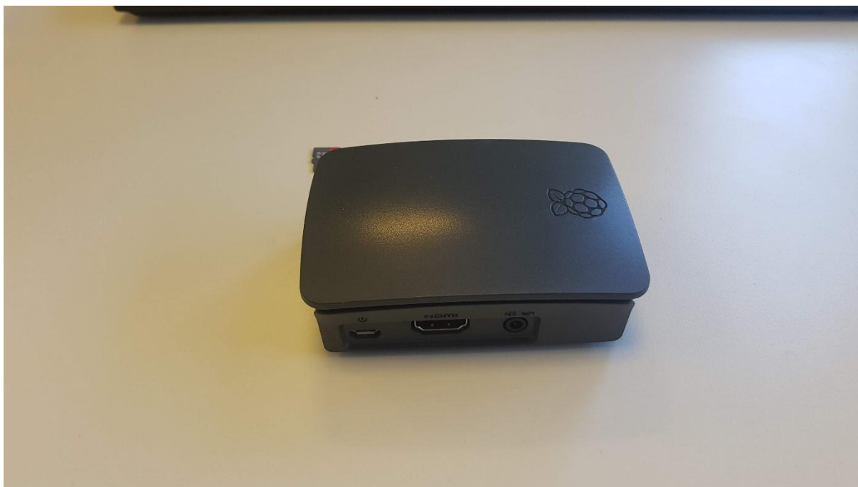
Figure 7. Attach the casing top cover
